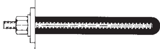
Untensioned dowels fully resin grouted.
