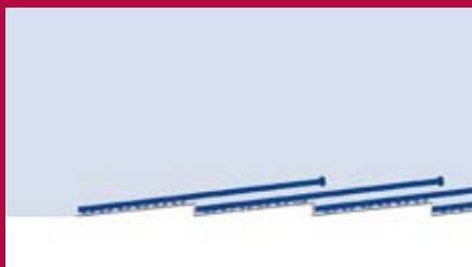
Single pipe umbrella support system with overlap to a double pipe umbrella support system
