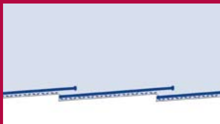
Single pipe umbrella support system with drainage
