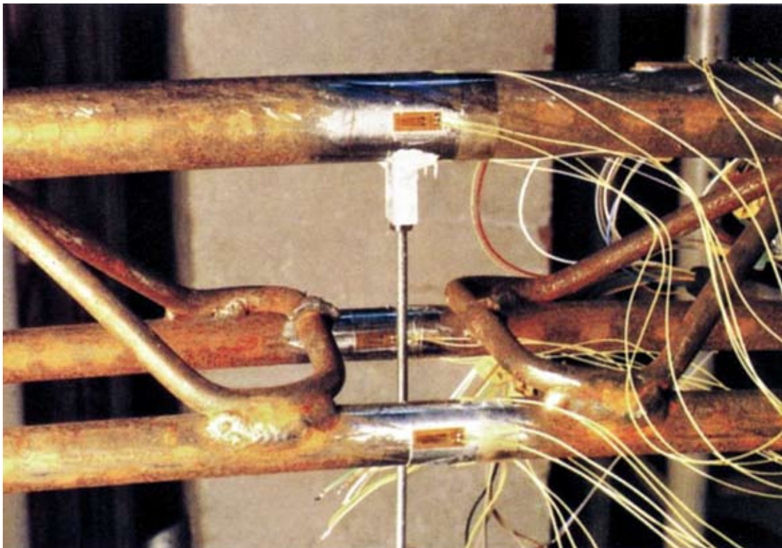
Experiments concerning the load-bearing capacity of lattice girders. Institute for Material Testing, Bureau for Civil Engineering, Technical University Munich.
