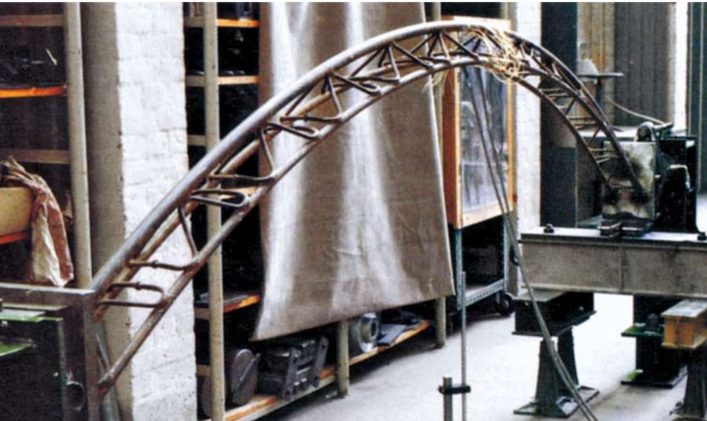
Experiments concerning the load-bearing capacity of lattice girders. Institute for Material Testing, Bureau for Civil Engineering, Technical University Munich.
