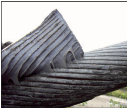
Adhesion of the tape on cable surface
